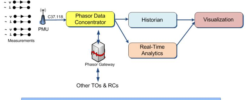
Gateways are used for external communications vis-à-vis ICCP for SCADA Systems
