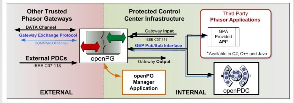
The openPG Manager allows all gateway inputs and outputs to be configured.
