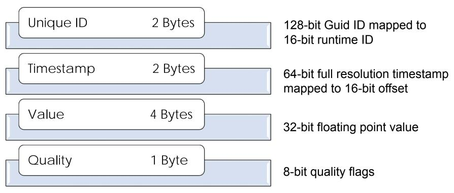
Several serialized measurements are grouped together to create a message payload. Total size is adjusted to reduce fragmentation.
