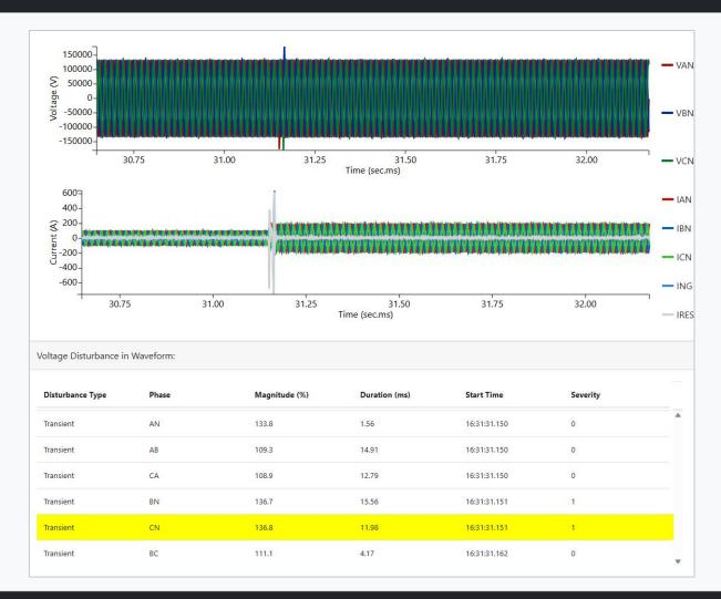
A **Transient** is a voltage disturbance that is very short-lived, identified by comparing a single sample to its counterpart in the previous cycle and flagging differences greater than 10% of nominal.
